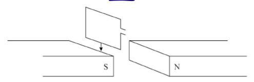
The coil is shown at four instants as it passes through the magnetic field.
